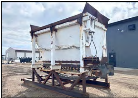
Clemro 3642 portable belt feeder, 14 yd. skid feeder, 36" discharge belt, hyd. tilting grizzly, 6" bar spacings
