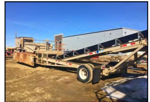
2012 Astec model 2148-50 truck unloader, cat C7 diesel power, electrical control panel
