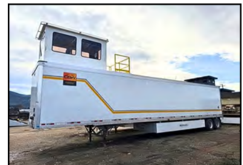
New 53 ft Great Dane, 6x11 control tower, side door and platform, under slung fuel tank, ready for electrical
