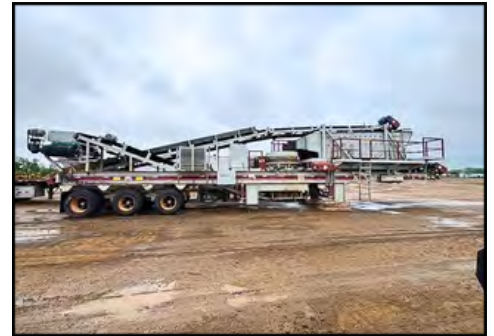
2008 Clemro XC1100 150 HP cone motor, 6x16 3 deck screen
