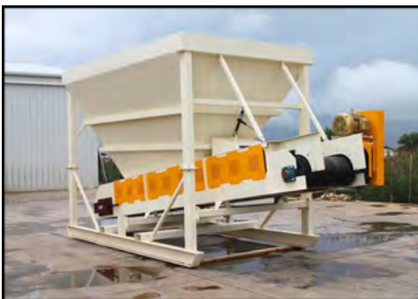
New 2026 14 yd. skid feeder, 36" vulcanized belt
