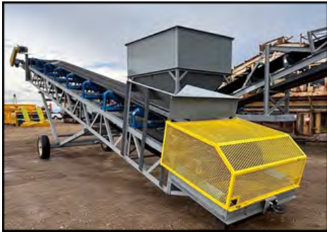
New 36" x 30 ft. pit portable stacker, chevron belt. #4 reducer, 10 HP 480 volt electric motor
