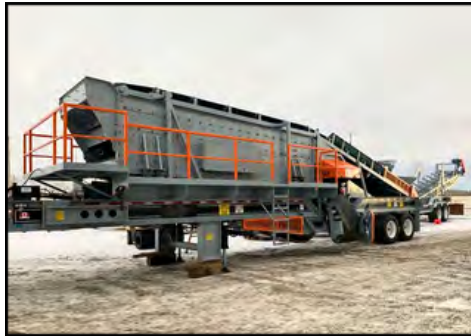
New 6x20 3 deck screen O/H feed belt, (2) cross conveyors, 100 ft cord pkg.
