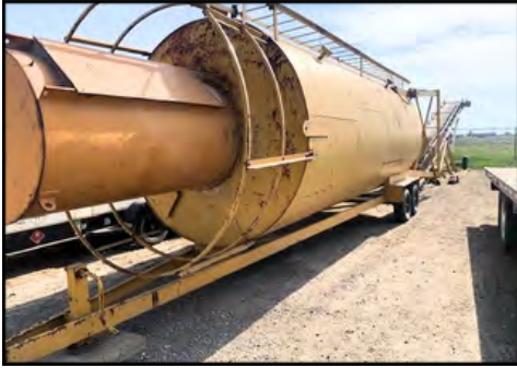
270 BBL Portable Belgrade cement silo, 8'-6" diameter, 36' overall length, Baghouse dust collector, Hi/Lo indicator lights, discharge auger, location Calgary
