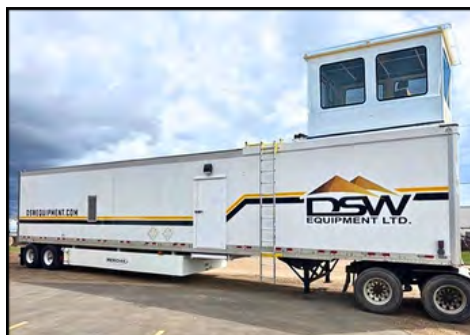
New 2026 build, A/B electrical, 1200 main, 38 stations, (3) VFD's 400 HP soft start, 6x11 control tower, under slung double walled fuel tank
