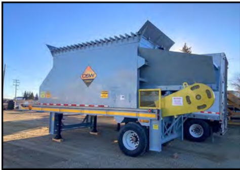
2023 Fasoli 14 yd. 36" Portable belt feeder C/W hyd. tipping grizzly
