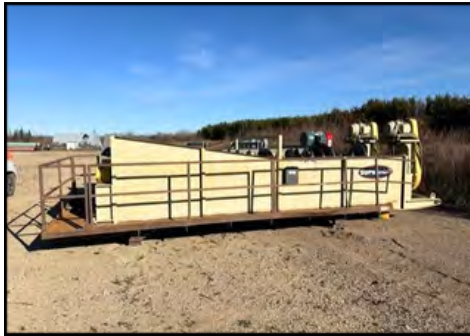
2019 Superior Blade Mill twin 44" x 20 ft. tub, (2) 30 HP 480 volt electric motors, power cords
