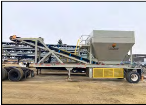
2008 Hikon 30 yd. surge bin, 42" discharge conveyor, 40 HP electric motor, fresh safety
