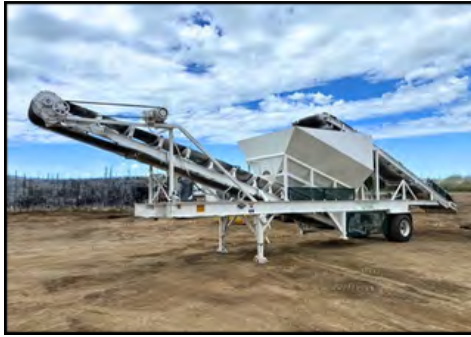
Mormak 20 yd. surge bin, 42" feed and discharge conveyor, single axel dual wheels, brakes & lights
