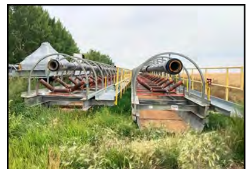
200 Ft of 54" Transfer conveyor, (4) 40 ft. Sections, (2) 20 ft. head & tail sections, 25 HP 480 volt motor, frame work for conveyor cover, spray bar system
