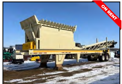
2011 Nor-Tech 3642 belt feeder, hyd. tipping grizzly with adjustable bars
