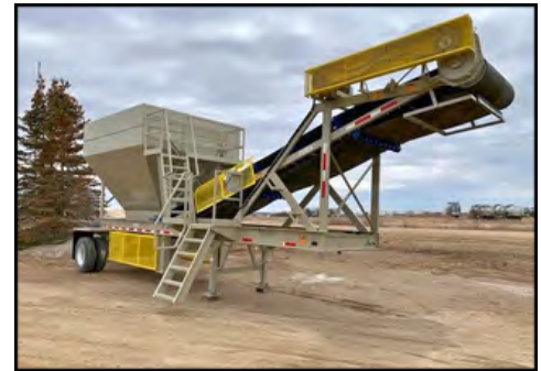
New Hikon 30 yd. surge bin. 48" discharge conveyor, 100 ft pwr.cord with plug end
