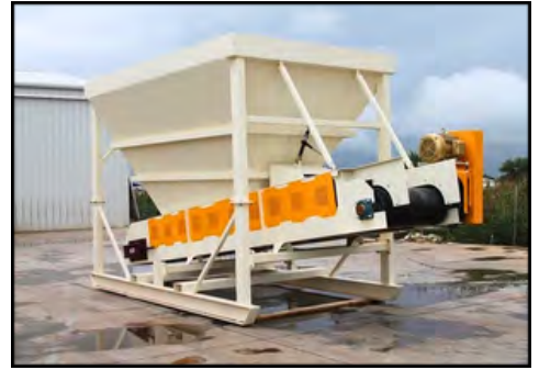
New 2026 14 yd. skid feeder, 36" feed belt, 100 ft power cord
