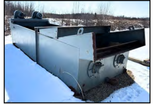
2018 Gator Twin 36" coarse material washer
