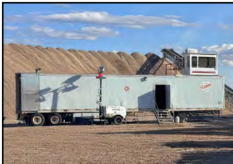
2008 53 ft, power van, A/B electrical, Cat C15 410 KW gen set
